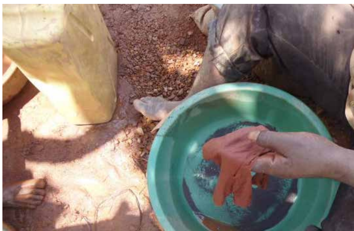
Fine materials of impurities that remain at the bottom of the basin after decantation
