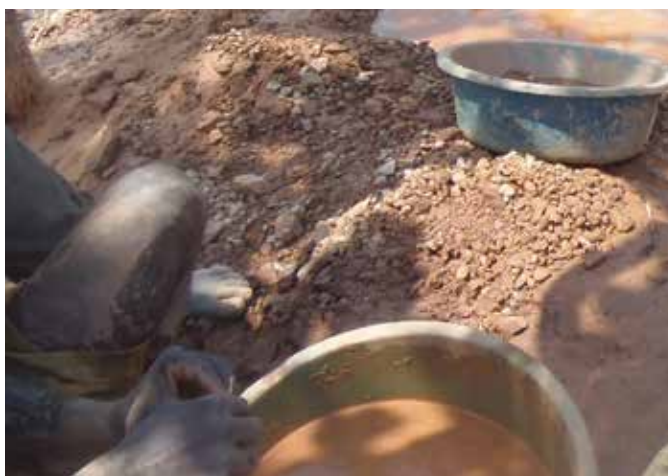
A miner soaking soil in water to extract gold from the mud.
